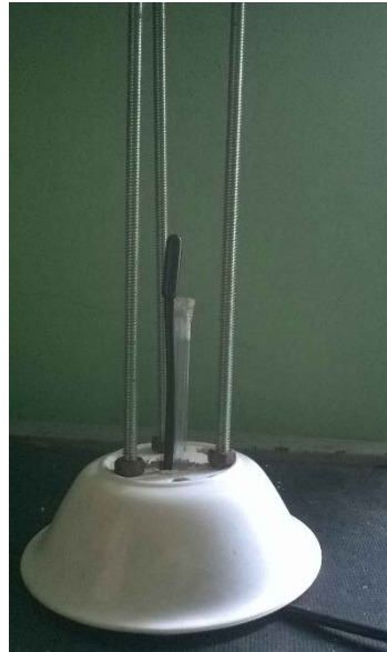
Figure B.7 Fix thermistor and other cups
