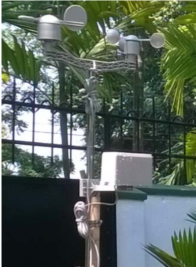
Figure 1 Mounting the Wind speed, Direction meters and Rain Gauge
